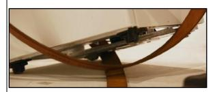
**STEP 1:** Tilt the item to one side and lay one strap diagonally on the floor beneath it with the buckle to the front of the item. Repeat this step to the other side to position the second strap.
